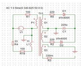
Medium E-I transformer 15 / 0 /15 V @ 150 VA 13.8 V for radios to 50 W
