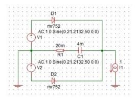
The Regulator acts like a Current Sink to the capacitor. There will be a little loss R1 in a capacitor.
