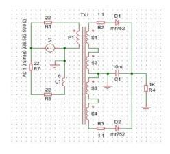
Large Toroid transformer 2 x 0 / 35 V @ 300 VA Current source for Peltier oven
